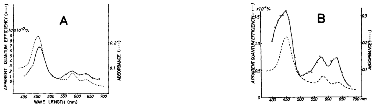
Fig. 3 Action spectra of the photogalvanic effect at the Pt-MgTMePyP electrode and the absorption spectra of the MgTMePyP aggregate deposited on a quartz plate (see Text). A and B: For the cells (1) and (2), respectively (see Text).
